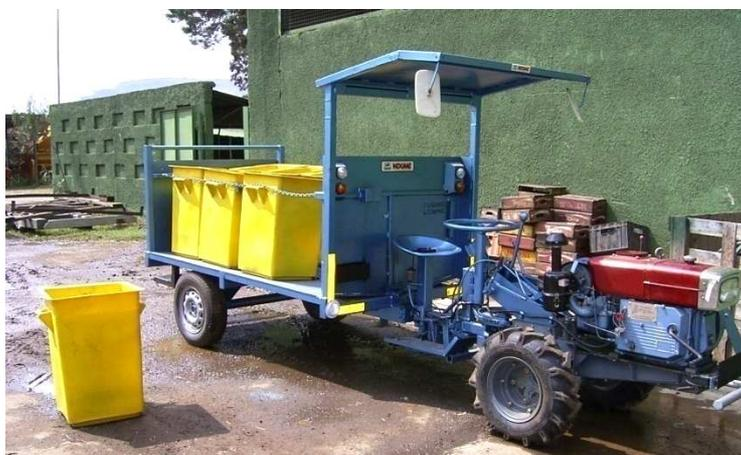
Figure 33 The UN-Habitat 2 wheel tractor solid waste transporter (10)
