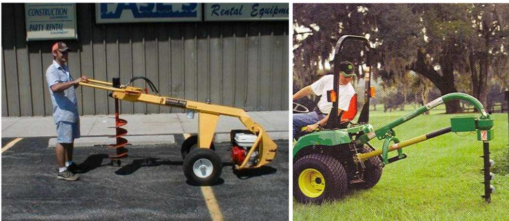
**Figure 33 showing two auger based drilling machines (15) (16)**
