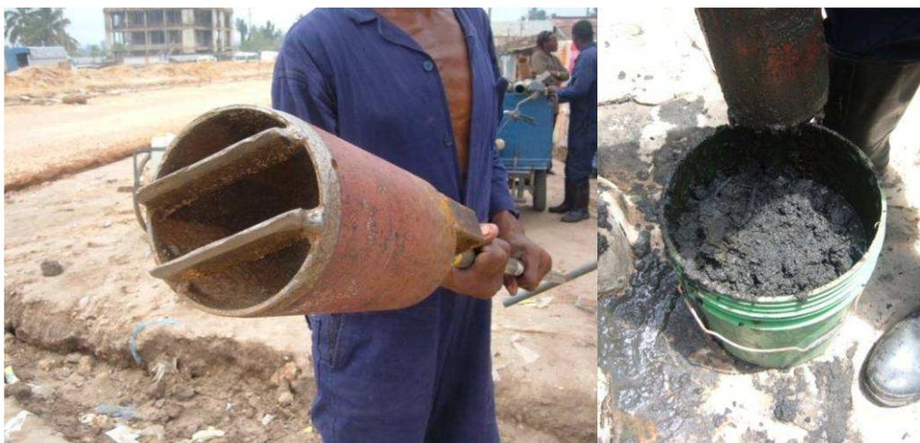
Figure 7 Image showing the Corer (4)
