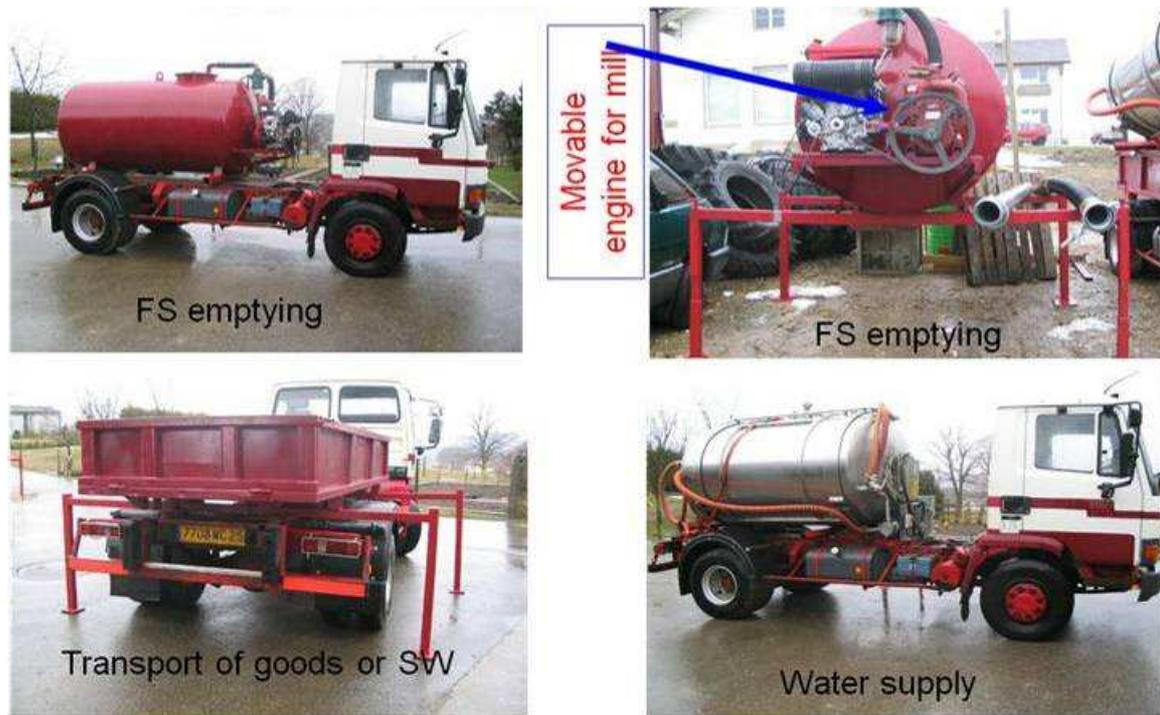
**Figure 35 showing one truck which is used for refuse collection, water delivery, and vacuuming (7)**
