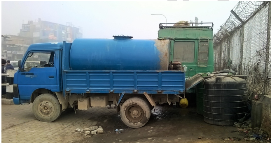
Figure 10: Faecal sludge collection from a mobile toilet
