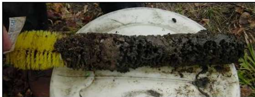
Picture 10 Particle filters to protect the infiltration system.
