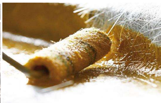
Picture 2 Lamination process from fiber enforced plastic
