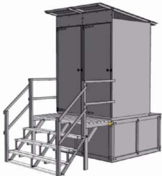
The cost of a double cubicle raised latrine is £450 and supplied through the [Oxfam procurement centre](#) in multiples of 6. Each twin latrine has a holding tank of 2m<sup>3</sup>.
