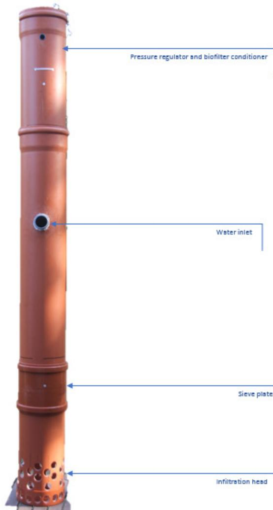
Figure 2 The Infiltration Column without the ventilation on top
