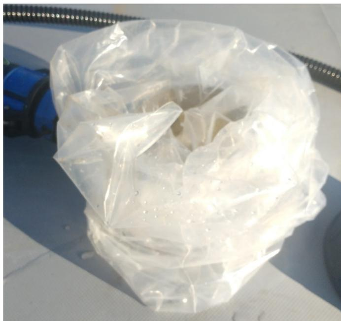
Figure 23 Bristle filter and flange covered with protective bag
