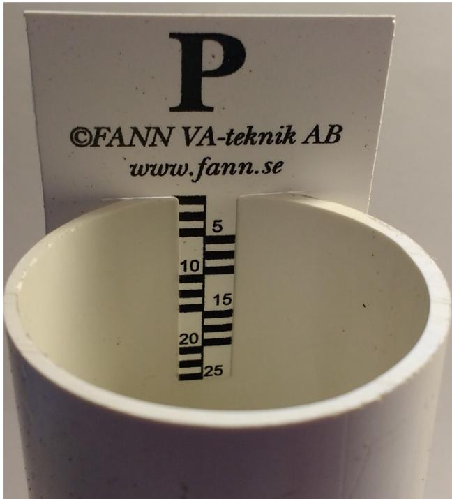
5. Place the holder with the sample tube in the bowl and fill the bowl with water until it comes out the overflow hole. Fill the sample tube with water until it overflows.
