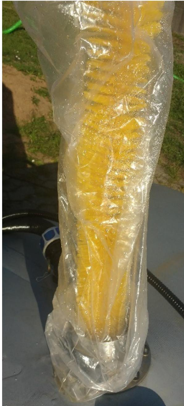
Figure 25 Filter in protective bag after removal from tank
