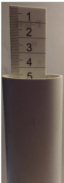
4. Place the level stick on the upper edge of the sample tube, so that the scale hangs inside the tube.
